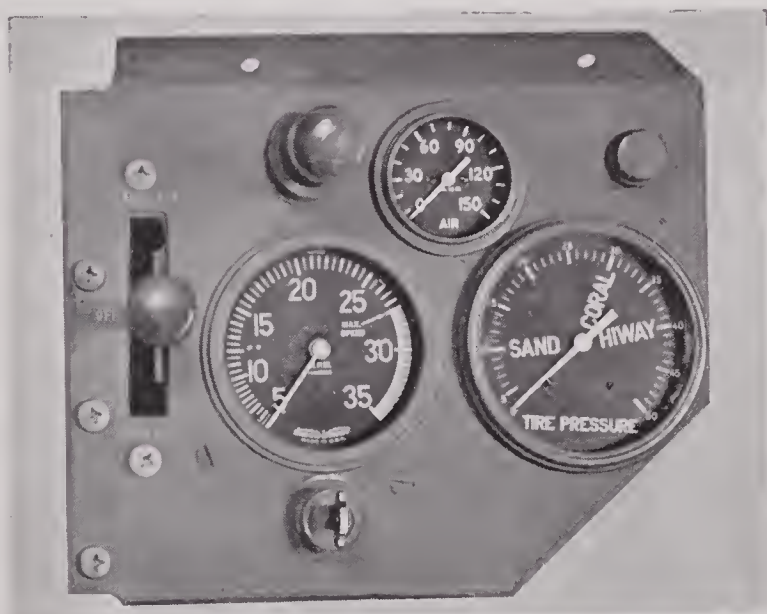
FIGURE 31. Dashboard controls for central tire-inflation system.
